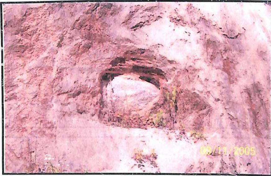
Plate No. 20: Corestone in the weathered rock
