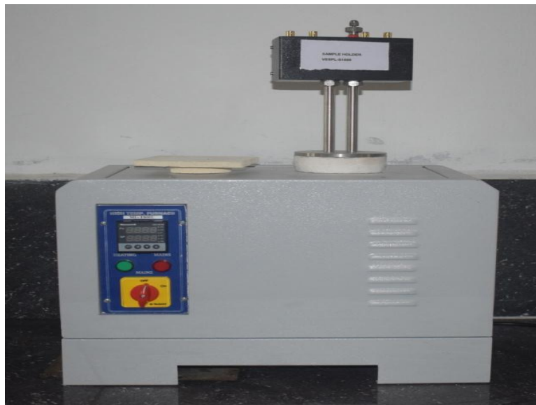
Fig. 2.4(a) High Temp Furnace with Sample Holder
