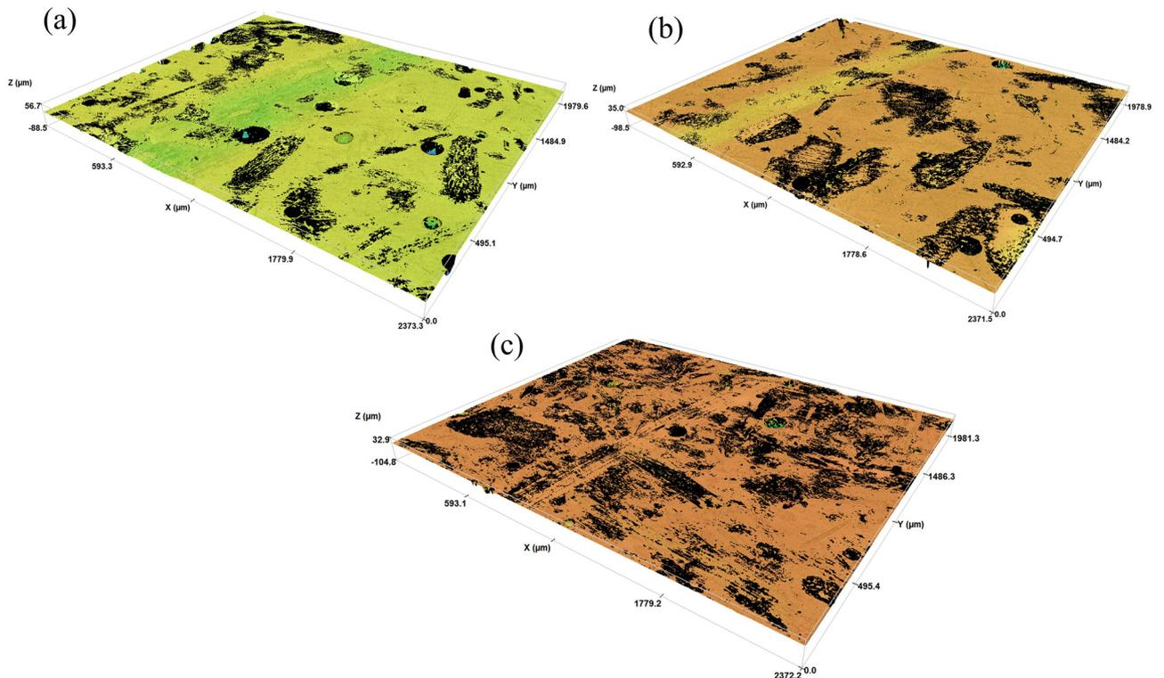
**Figure 4:** Surface profile images of the matrix with wt.% of (a) 5% ( $R_a = 0.15 \mu\text{m}$ ,  $R_t = 4.59 \mu\text{m}$ ), (b) 15% ( $R_a = 0.35 \mu\text{m}$ ,  $R_t = 6.69 \mu\text{m}$ ), and (c) 25% ( $R_a = 1.15 \mu\text{m}$ ,  $R_t = 11.5 \mu\text{m}$ ) BF content.
