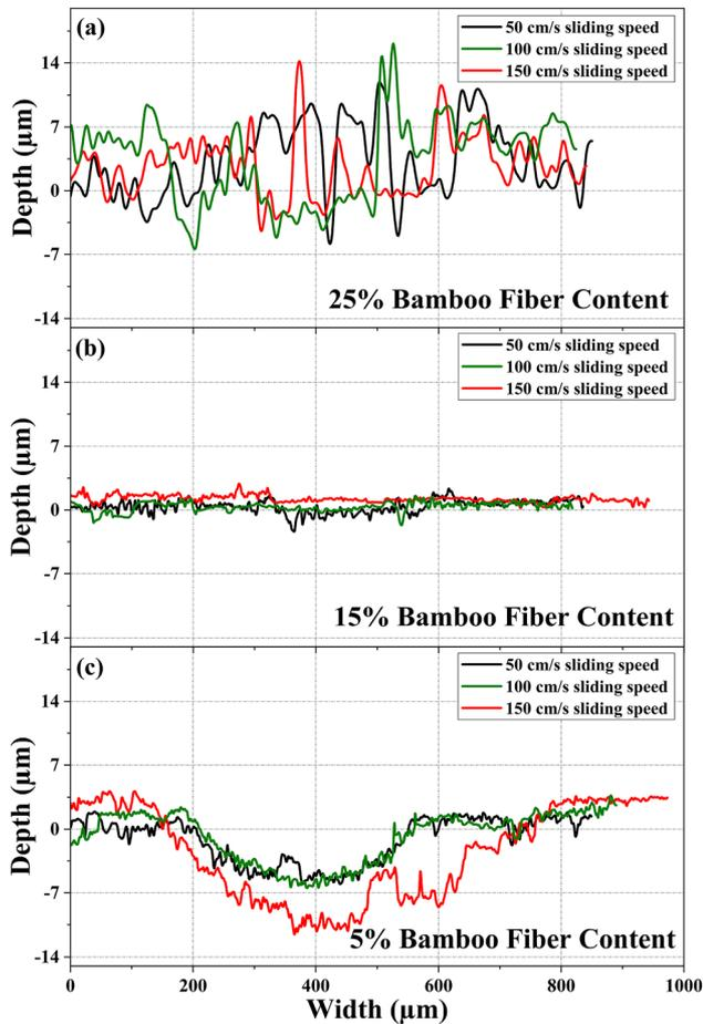
Figure 5: Surface profile graphs of test path for tribology tests performed at 5 N load with (a) 5 %, (b) 15 %, and (c) 25 % BF content.
