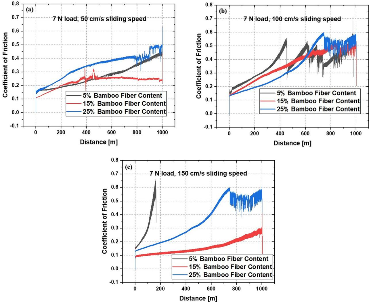
**Figure 10:** COF versus travelled distance for the tribology tests performed at 7 N load for sliding speed at (a)  $50 \text{ cm s}^{-1}$ , (b)  $100 \text{ cm s}^{-1}$ , and (c)  $150 \text{ cm s}^{-1}$  BFC composite materials.
