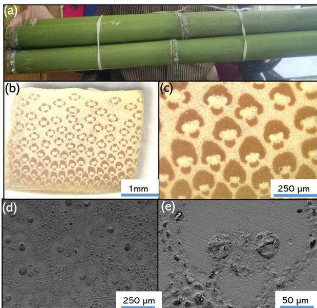
**Figure 1:** Microstructural Analysis of Bamboo Fibers. (a) Bamboo culm, (b) cross-section of bamboo culm, (c), (d) vascular bundle of the BF under optical microscope and FE-SEM, and (e) elementary BFs and vascular bundle under FE-SEM.
