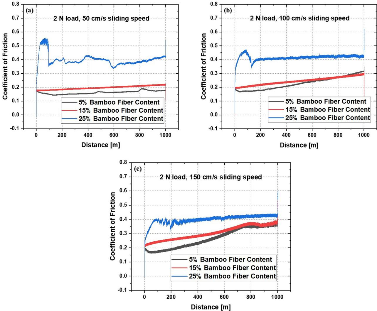
**Figure 8:** *COF* versus travelled distance for the tribology tests performed at 2 N load for sliding speed at (a)  $50 \text{ cm s}^{-1}$ , (b)  $100 \text{ cm s}^{-1}$ , and (c)  $150 \text{ cm s}^{-1}$  BFC composite materials.
