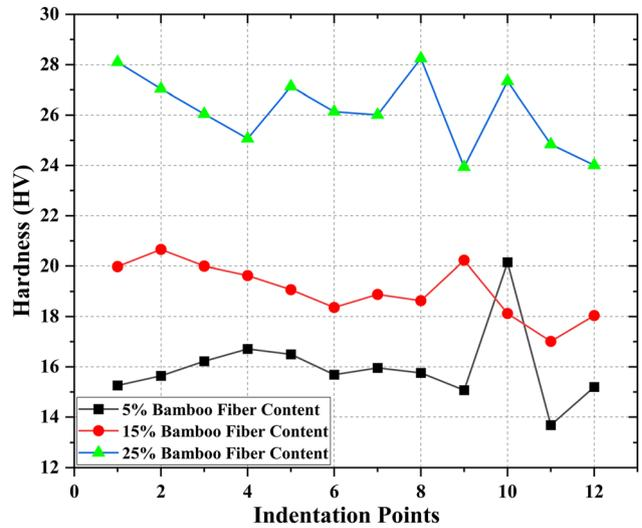
Figure 7: Hardness graphs of matrix surfaces with (a) 5 %, (b) 15 %, and (c) 25 % BF content.
