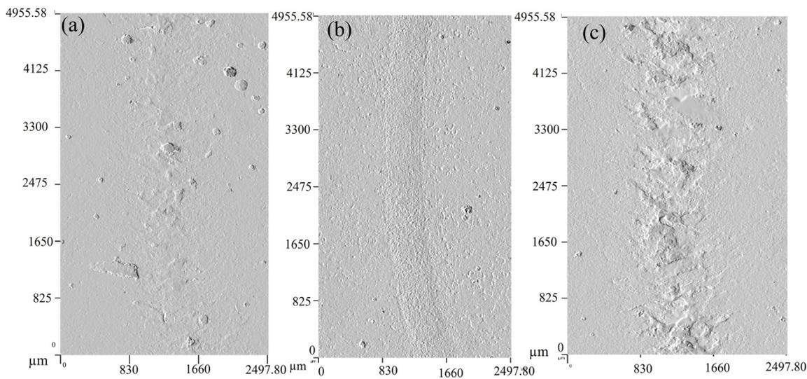
Figure 6: 2D surface profile images of tribology test path: (a) BFC 5,  $R_a = 5.28 \mu\text{m}$ , (b) BFC 15,  $R_a = 2.35 \mu\text{m}$ , and (c) BFC 25 BF content,  $R_a = 17.57 \mu\text{m}$  for tribology test performed at 7 N load and  $150 \text{ cm s}^{-1}$  sliding speed.
