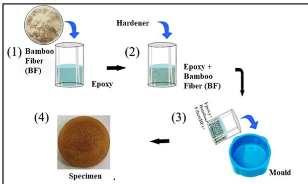
**Figure 2:** Flow chart of epoxy-based matrix preparation with BF content.
