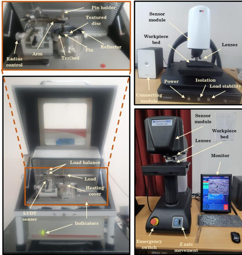
**Figure 3:** Experimental setup for surface profiling, hardness tests and tribology tests.
