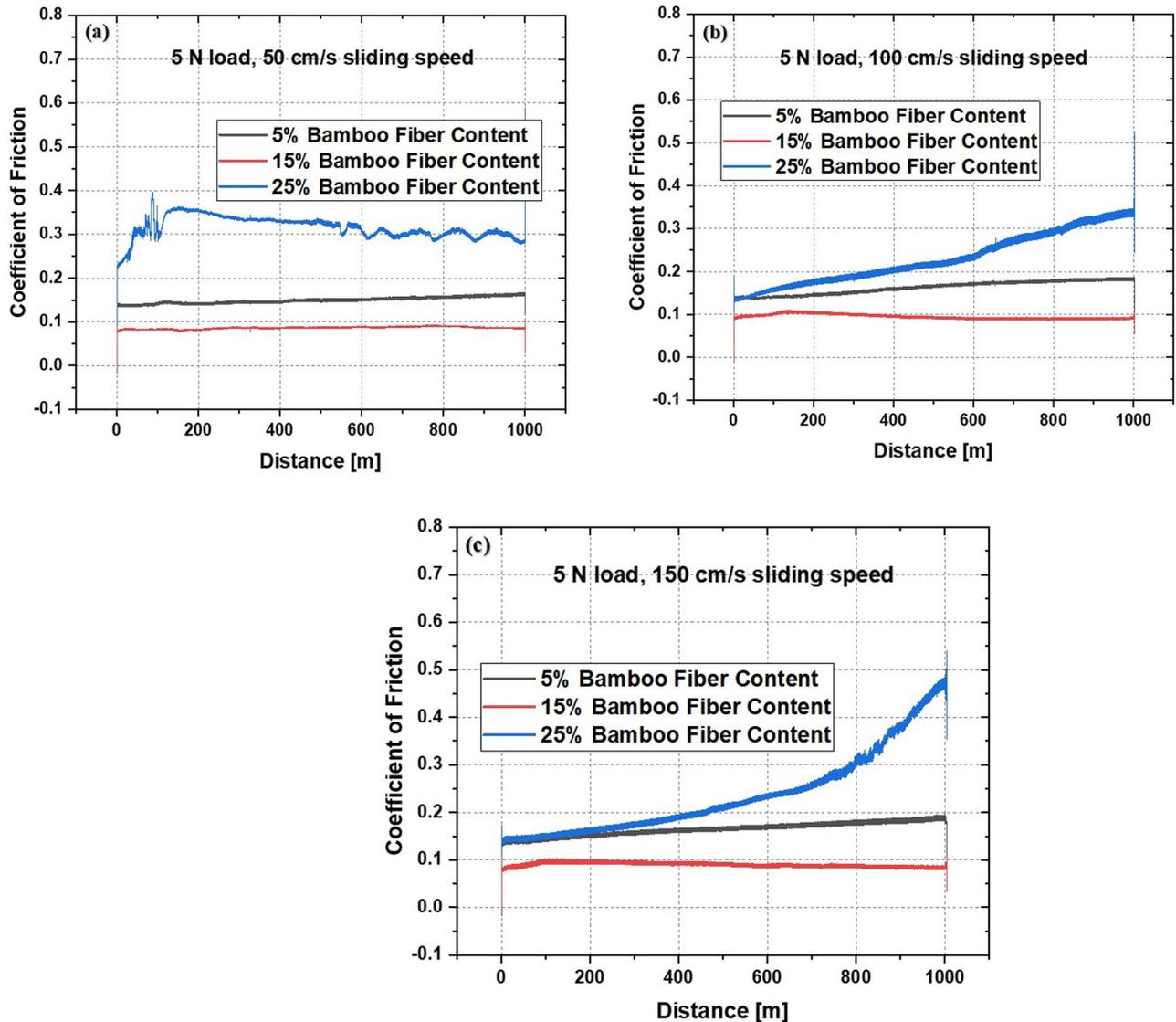
**Figure 9:** COF versus travelled distance for the tribology tests performed at 5 N load for sliding speed at (a) 50 cm/s, (b) 100 cm/s, and (c) 150 cm/s BFC composite materials.
